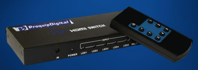
The 5 in 1 HDMI switch routes high definition video (in multiple resolutions up to 4Kx2K) and digital audio from any one of the five sources to one HDTV.
