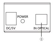
① TOSLink(Optical Fiber) Input Port: Connect the TOSLink input port to the TOSLink output port of audio equipment such as audio amplifier,AV receiver or DVD player.
