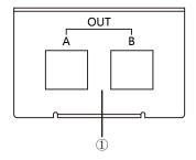
① TOSLink(Optical Fiber) Output Ports A and B: Connect the TOSLink output ports to the TOSLink input port of audio equipments such as audio amplifier and AV receiver.
